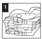
To move the recline foot to the forward-facing position, lay restraint on it's side.
